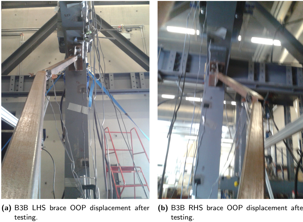
Figure 5.24: B3B OOP displacements after testing
