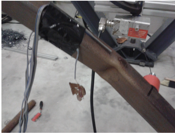
Figure 5.16: Local buckling in the B3A RHS brace.
