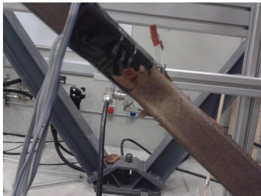
Figure 5.13: Necking of RHS brace during B2B testing.
