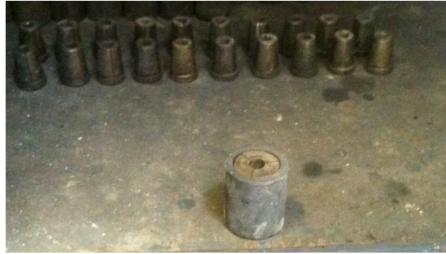
Figure 4.5: PT anchorage system used in test frame.
