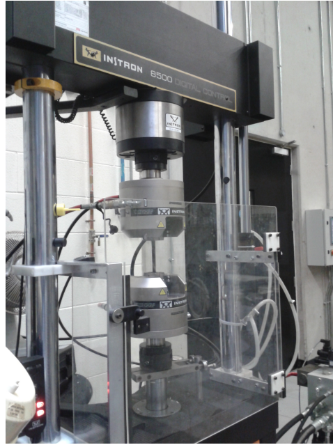
Figure 5.1: Instron 8500 Digital Control Test Machine.
