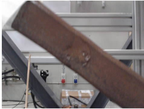
(b) B4B RHS brace local buckling.
