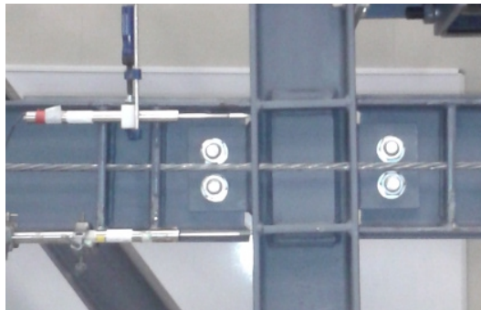
Figure 5.4: LVDT instrumentation on upper beam-column connection.
