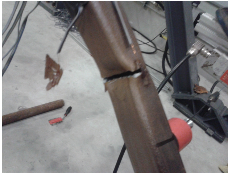
Figure 5.17: Fractured B3A RHS brace.
