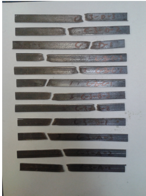
(b) Fractured C2 specimens.
