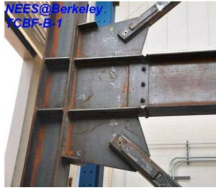
Figure 4.3: Typical connection of brace gusset plate to beam-column connection [79].
