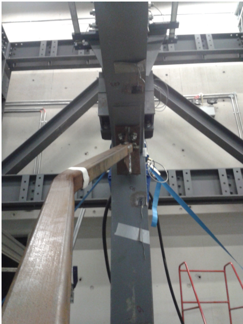
(a) B4B LHS brace OOP displacement after testing.
