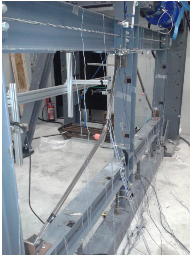
Figure 5.8: Buckling out of plane of the B1A specimens.
