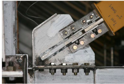
Figure 4.4: Beam-only gusset plate connection presented in Berman and Bruneau [10].
