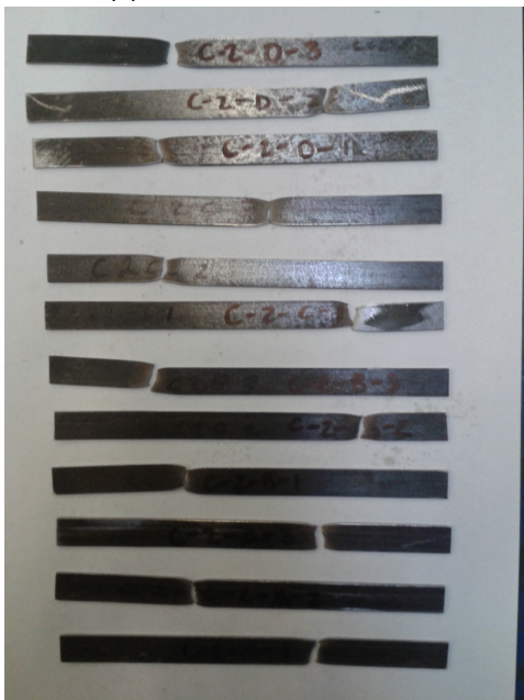
(c) Fractured C3 specimens.
