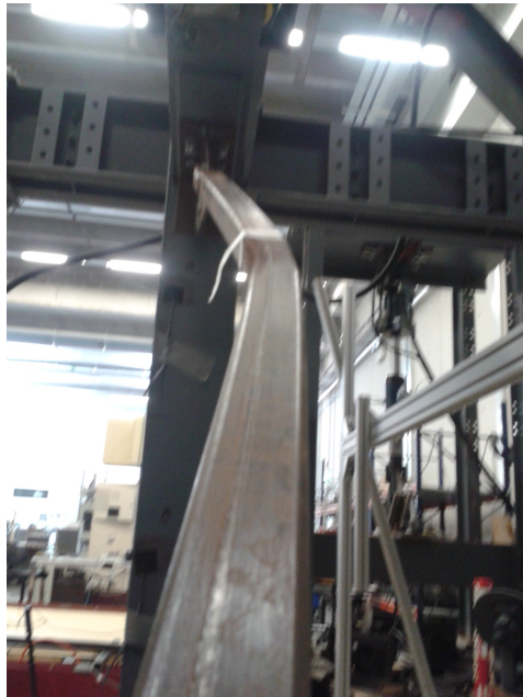
(b) B4B RHS brace OOP displacement after testing.
