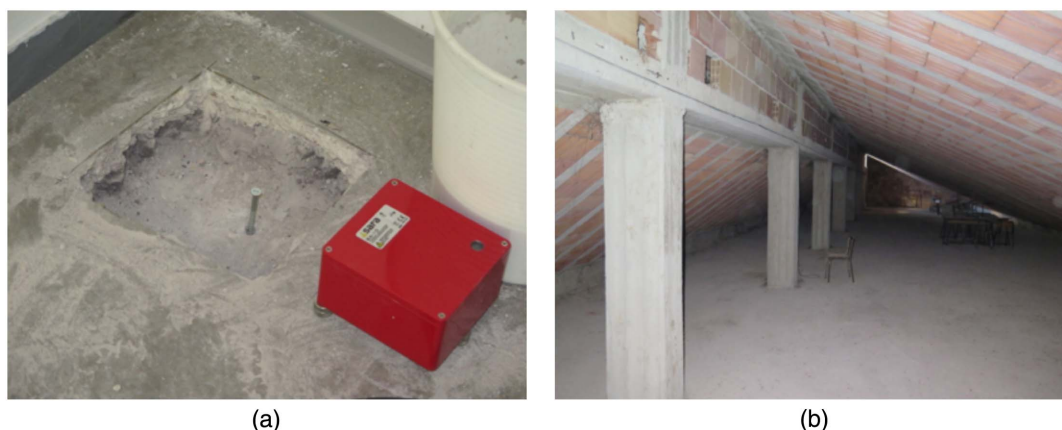
Fig. 3. Accelerometer installation for Ancona school building: (a) reference accelerometer at slab on grade; and (b) top floor slab location of accelerometers for dynamic identification.
