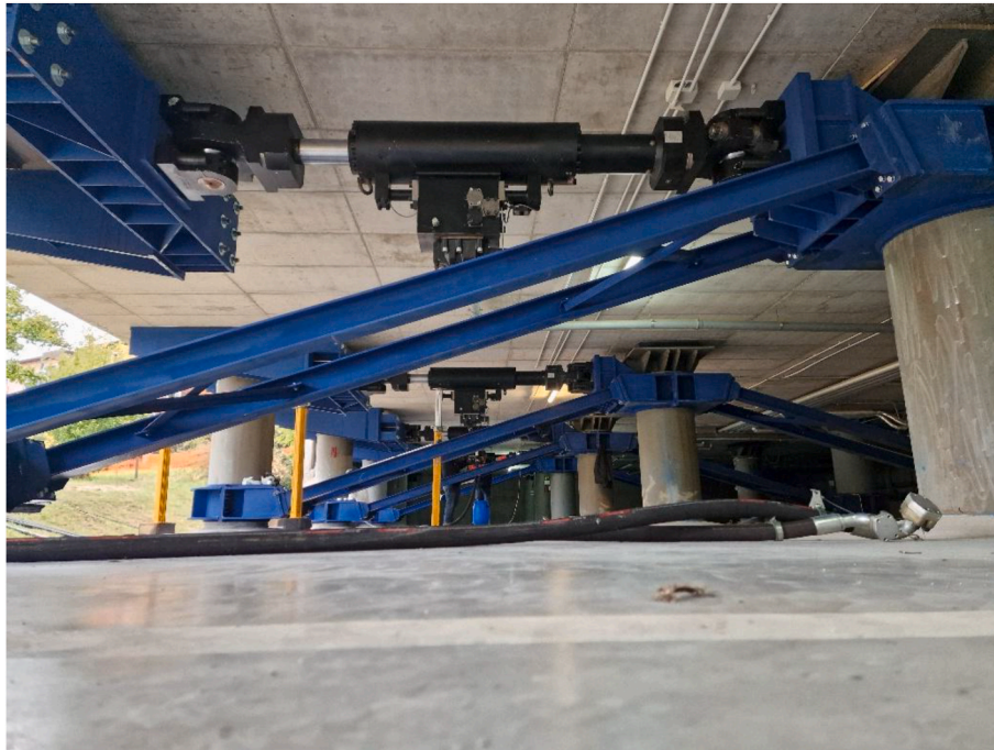
Fig. 7. Actuator installed on reaction frame.
