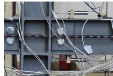
Figure 6 LVDTs for measuring rocking connection gap-opening
