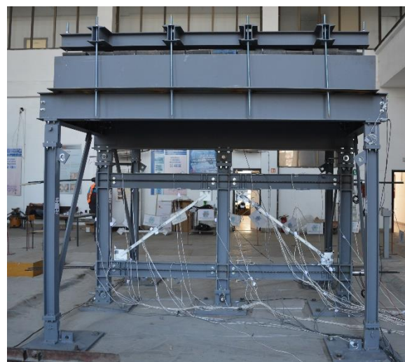
Figure 2 Overview of SC-CBF structure (on shake table)
