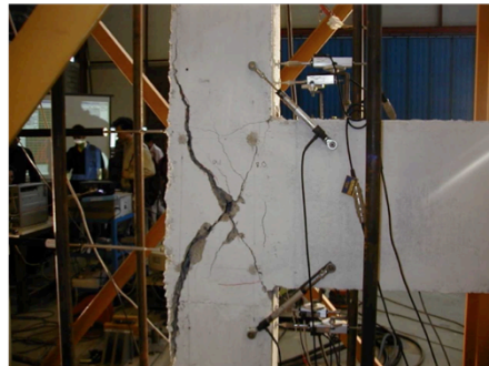
(b) Diagonal cracking in joint.
