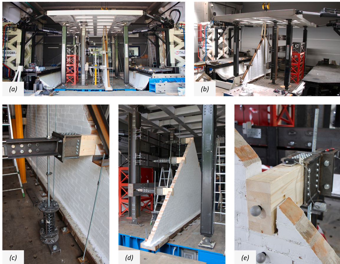
Fig. 3. Testing setup photos and details: (a) frontal view of the 9D dual shake-table system; (b) lateral view of the same system; (c) loading arm connected to spring device; (d) gable specimen with loading frame and instrumentation frame; (e) timber purlin seated in masonry pocket.
