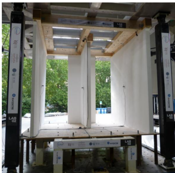
Figure 4- 9DLAB shaking-table facility at Eucentre with the gypsum partition specimens installed between the lower and upper tables.
