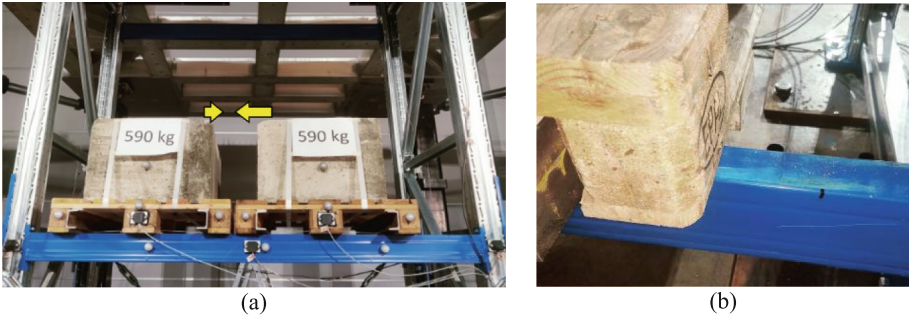
Fig. 7. Final pallet positions after biaxial test #12: (a) down-aisle sliding and (b) surface wear on the steel beams.
