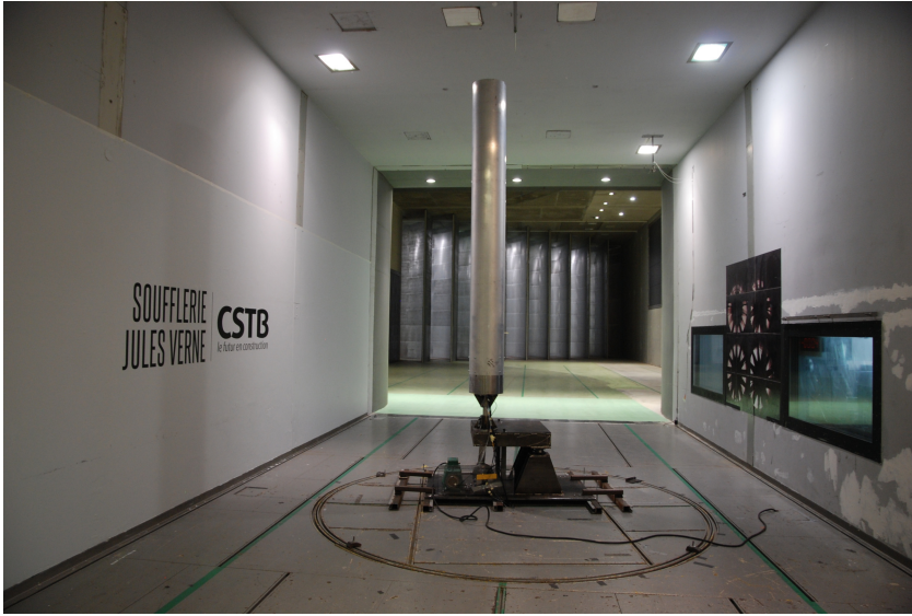
Fig. 2. Wind tunnel setup with one isolated cylinder mounted on the tilting table.
