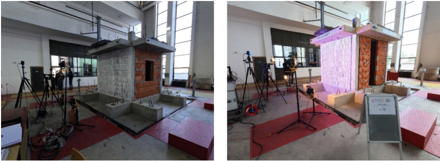
Fig. 8. DIC setup Model 1 and Model 2.
