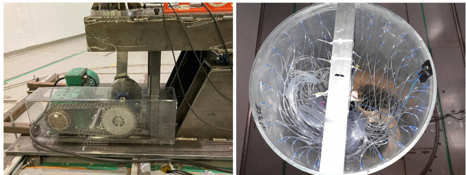
Fig. 3. Detail of the tilting table and of the sensor installation from the top of cylinder.
