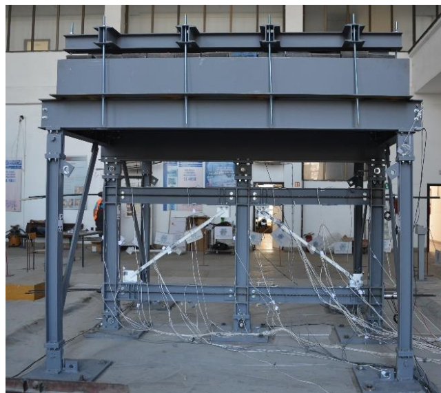
Figure 3: Overview of the IZIIS shake table test set-up of the SC-CBF system (Goggins et al. , 2021)
