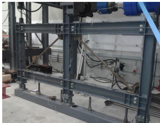
Figure 2: The SC-CBF tested in the large structures laboratory, University of Galway (adapted from O'Reilly and Goggins 2021).
