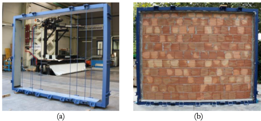
Figure 2. (a) Structural frame; (b) masonry infill at the end of the construction (Kurukulasuriya et al. , 2023).
