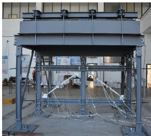
Figure 2 Overview of SC-CBF structure (on shake table)
