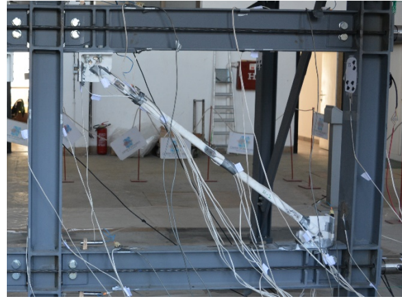
Figure 5 SHS brace specimen and gusset plates (B40x40, north bay)
