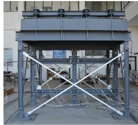
Fig. 8 – Overall view of the SC-CBF system (north direction is from left to right)
