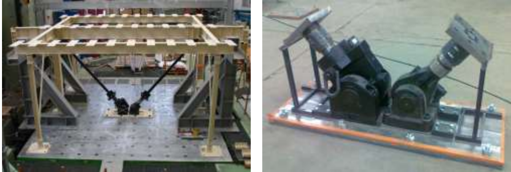
Figure X.2. Test frame without added masses and MTS swivel bearing with load cells
